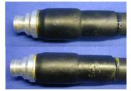
Because of too much heat or not enough movement of the heat source the sleeves are damaged (burned).
